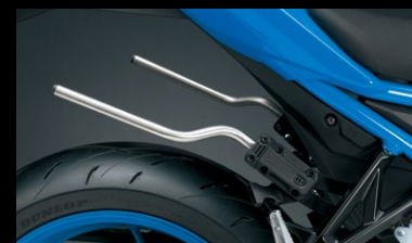
Side Case Bracket Set 93700-25840-000 This bracket set is required for installation of soft side case set. Set of right and left side.
